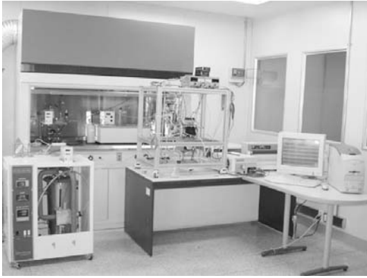
Fig. 2 A schematic diagram and photo of experimental apparatus to measure two-phase flows in a multi-channel
